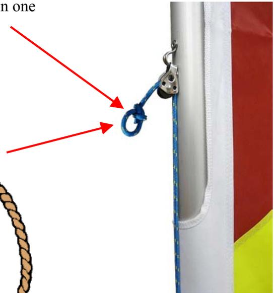
Thread through block (pulley) on front of mast. Lead down to and through cleat. Tie another bowline (3 – 5" diameter) to use as a handle.
