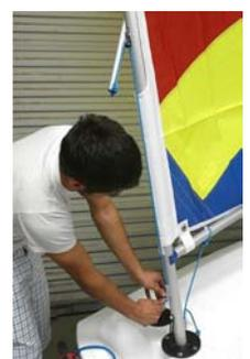
11. Attach tiller to rudder. Sandwich rudder blade between spread tiller forks. Make sure extension is on top, per photo. Secure with two bolts.
