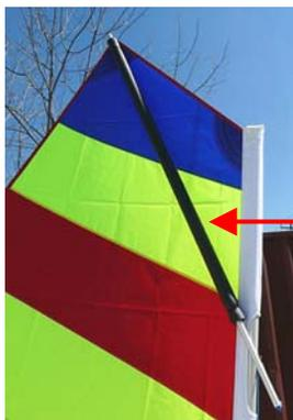
Slide a section of pool noodle or Pipe insulation over the upper end of the sprit to help prevent turning turtle in event of capsiz.
