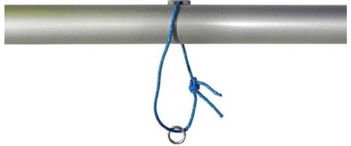
7. Rig outhaul. Tie a figure eight knot (stopper knot) in one end of outhaul line. Thread through outhaul fitting in end of boom, pass through grommet in sail, back through outhaul fitting, then lead to cleat. Tie a bowline in end for a handle.
