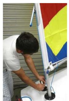
11. Attach tiller to rudder. Sandwich rudder blade between spread tiller forks. Make sure extension is on top, per photo. Secure with two bolts.
