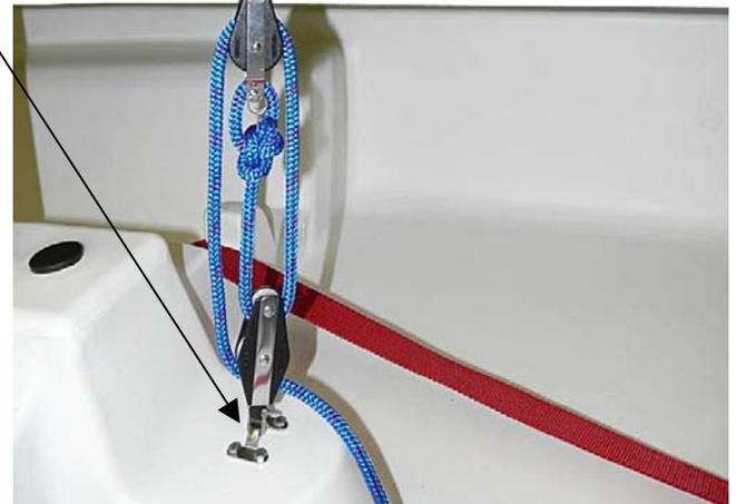
10. Attach sprit. Put one end of sprit into loop at peak (top corner) of sail. Push the sprit up and out until you can hook the other end into the small bowline of sprit adjuster. Pull sprit adjuster line below cleat to tighten. Tighten just until diagonal wrinkles disappear from sail, then cleat line.
