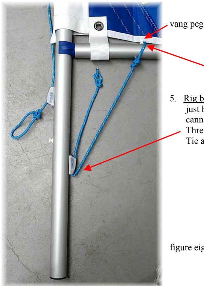
5. Rig boom vang. Tie a bowline very snugly around boom just behind vang peg. It should be tight enough that it cannot be easily slid over vang peg. Thread other end into vang cleat from the bottom. Tie a figure eight knot in the end.
