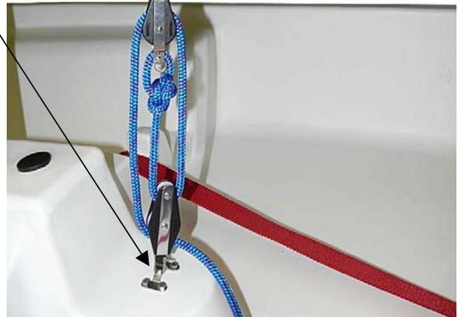
10. Attach sprit. Put one end of sprit into loop at peak (top corner) of sail. Push the sprit up and out until you can hook the other end into the small bowline of sprit adjuster. Pull sprit adjuster line below cleat to tighten. Tighten just until diagonal wrinkles disappear from sail, then cleat line.
