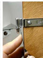
**Daily unrigging:** When finished sailing for the day simply unhook the mainsheet at clip. Remove sail and lay on ground. Remove sprit and lay it next to mast. Fold peak of sail down to mast. Fold boom up to mast. Roll mast boom and sprit into sail.
