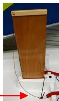
Add a piece of 1/8" x 52" line to daggerboard so it can be tied into boat and not float away.
