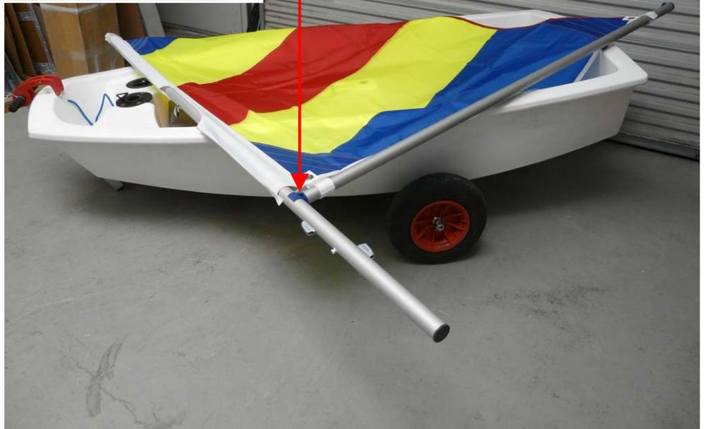
4. Rig sprit adjuster. Tie a very small bowline (1" or less diameter) in one end of sprit adjuster line.
