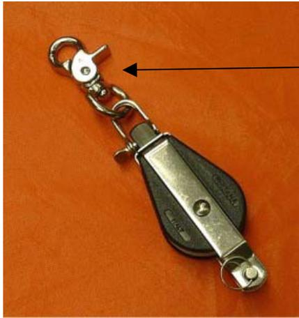
Install trigger shackle at top of becket block.
