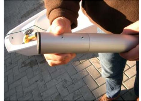
Apply a heavy coating of silicone sealant to mast extender in an effort to make a watertight seal with mast and to keep it attached. Slide together and wipe off excess silicone.
