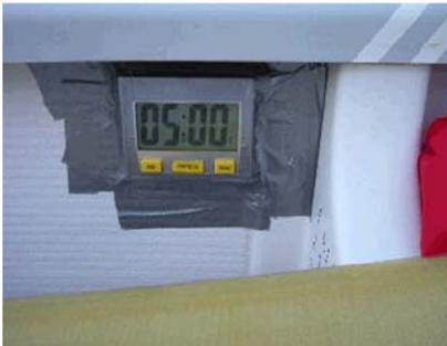
We have been concerned that the Velcro provided with the timer is not strong enough to withstand most capsizes. Here are two ideas that have worked well and provide great visibility of the timers for the time being. The first has the timer duct taped to the port sidewall. Not sure how effective this would be if you tried to port tack the fleet?
