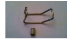
2. Once the handle is removed the only thing preventing the bailer slide from dropping out of the bottom is the 1/8 in. lip at the rear top of the bailer slide. Carefully use vise grips or pliers to bend it straight. If the bailer is down in a hole in the floor the lip maybe difficult to get at.
