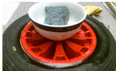
This tube tire leaked at the stem See the suds created by soap
