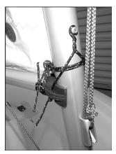
from the van. The bling fixes the inboard position of the boom on the mast and consequently the fullness or flatness of the luff. Without the bling, vang tension also affects the luff tension... By twisting the bling, the
