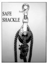
The mainsheet should be attached to the boom bridle with a shackle that is easy to use, lightweight, inexpensive, takes only one hand to use and is SAFE! Why one handed? So the sailor can steer while connecting or disconnecting.
