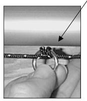
Next, secure to the aft bridle fitting with a trucker's hitch pull the trucker's hitch as tight as you possibly can. To finish it off, wrap the hitch with half hitches that draw it even tighter. Now pull the bridle like an archery bow string. If it pulls close to 10 cm, start over with the trucker's hitch and stretch it even tighter.
