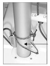
Most eight year olds are able to step the mast alone after a little practice. The trick is to keep the hands spaced wide apart on the mast and to work in harmony with the wind, not against it. If the rig must be transported any distance or if the wind is too strong, fold the boom up to the mast and carry it folded up.
