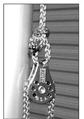
Rig the Sprit Adjuster: halyard, handle and block
