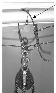
The **bridle preventer** should restrict the bridle to pulling no more than 10 cm from the boom in event it loosens. Tie with a sheet bend (a square knot would flip and loosen under tension).
