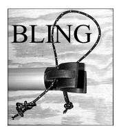
Starting with the boom jaws, tie the **boom "bling".** Tie a double figure eight knot close to one end (the double twist in the knot makes it far easier to untie in the future). Pass it through the holes in the gooseneck as shown and tie another figure eight knot in the end.
